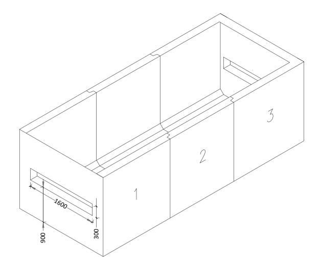
Isometric view precast chamber SCALE 1:50
